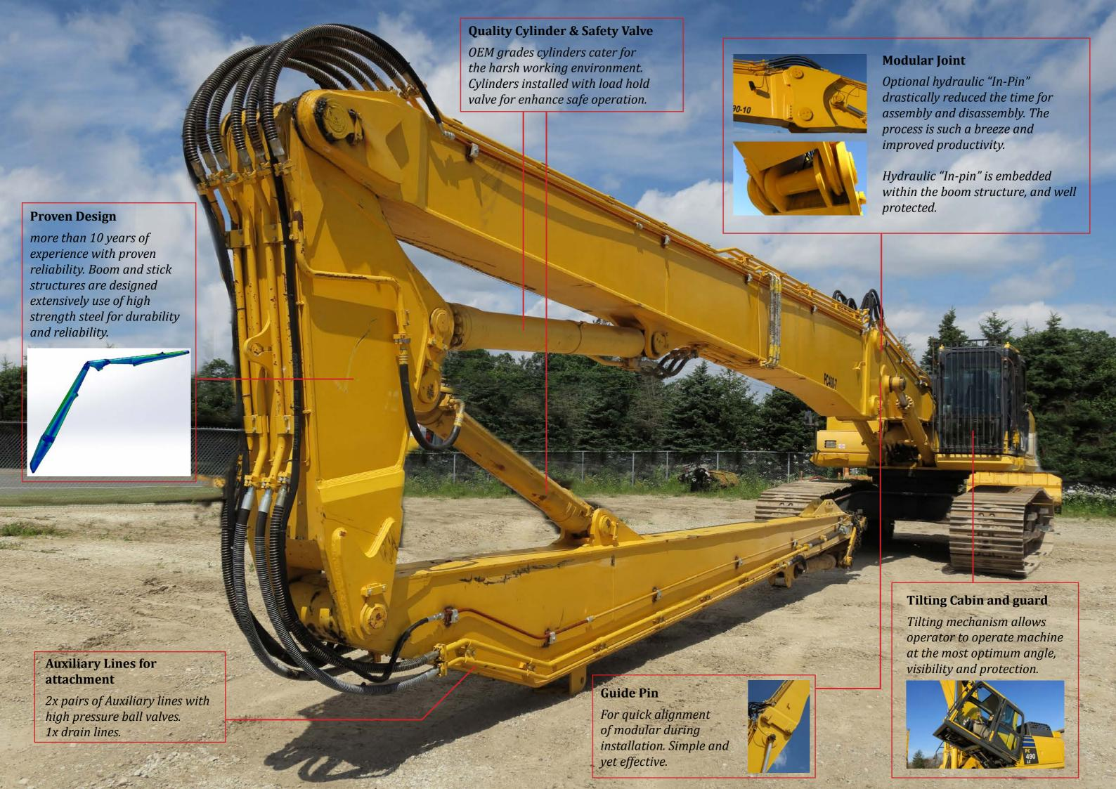
We design and customize demolition solutions for every make and model of hydraulic excavator, starting from 10 metric tons (22,000 lbs) mini-excavator and upward. Depending on your excavator size, the demolition boom can easily handle work tools ranging from 0.5 (1,100 lbs) to 4 tons (8,800 lbs) of weight.
