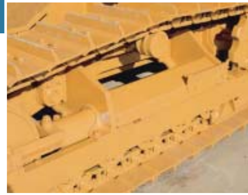
An easy access cleanout area makes undercarriage maintenance easier, saving valuable time.
