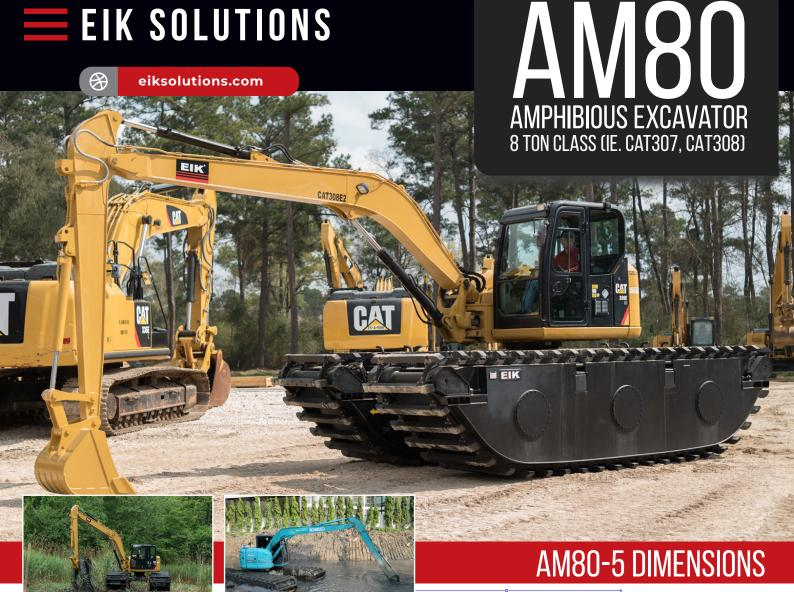
An amphibious excavator/marsh buggy is specifically designed to maneuver in marshland, swampy areas and soft terrain. It is completely self-propelled and can virtually access all terrains while requiring minimum supporting transportation and hoisting
