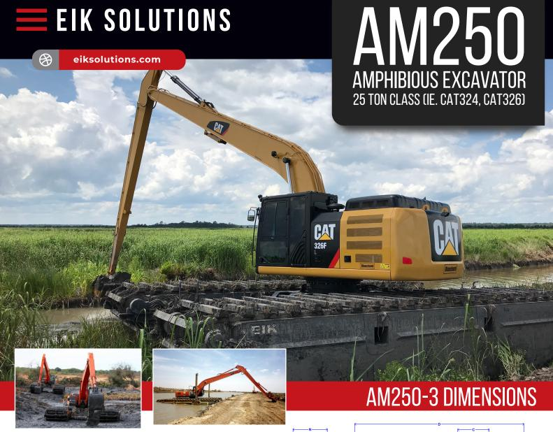
An amphibious excavator/marsh buggy is specifically designed to maneuver in marshland, swampy areas and soft terrain. It is completely self-propelled and can virtually access all terrains while requiring minimum supporting transportation and hoisting equipment.
