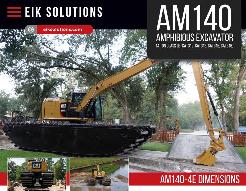
An amphibious excavator/marsh buggy is specifically designed to maneuver in marshy, swampy areas and soft terrain. It is completely self-propelled and can virtually access all terrains while requiring minimum supporting transportation and hoisting equipment.
